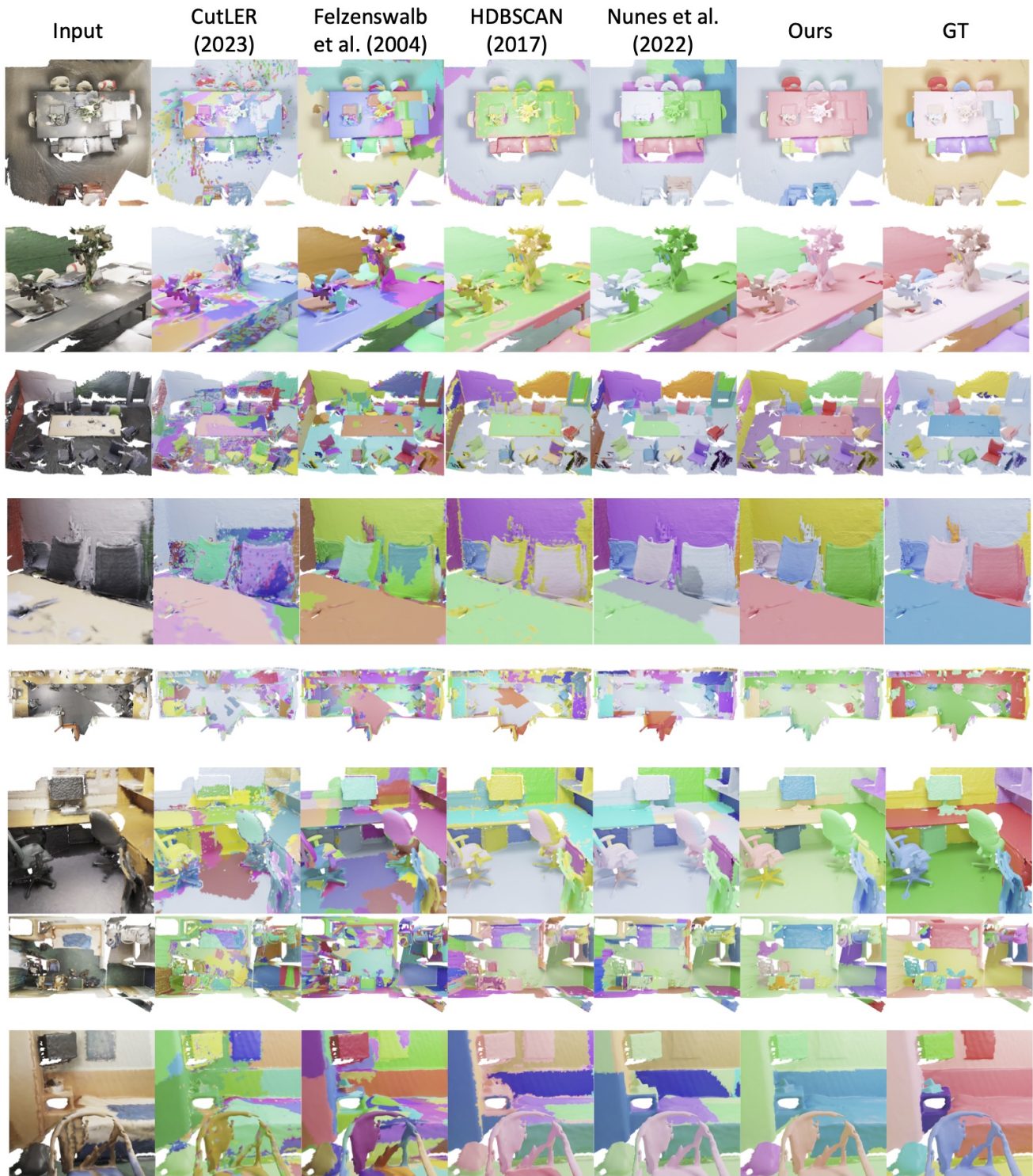
Figure 3. Qualitative comparison on ScanNet [9] scenes with projected predictions from the 2D method CutLER [52], traditional clustering-based methods Felzenswalb [14] and HDBSCAN [32], and the GraphCut-based cluster refinement method [35]. Our approach leverages strong pseudo mask prediction and a self-training strategy to produce cleaner, more accurate instance segmentation.
