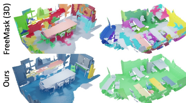
Figure 5. Initial pseudo masks generated by UnScene3D in comparison with a 3D-lifted FreeMask [51]. FreeMask tends to produce a larger set of noisier pseudo masks, while we rely on a cleaner but sparser set for our self-training.
