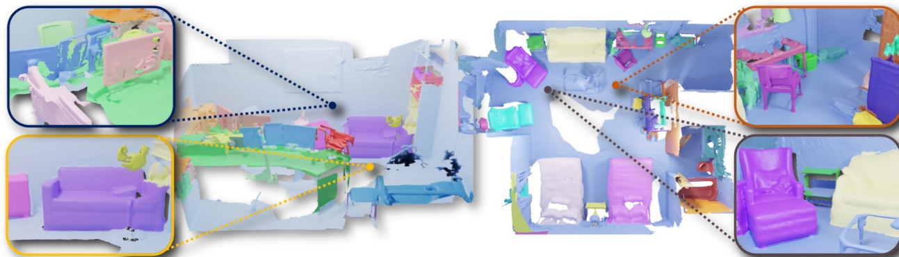
Figure 1. We propose UnScene3D, a fully-unsupervised 3D instance segmentation method, effectively separating semantic instances without requiring any manual annotations. We utilize geometric primitives to ensure crisp masks, and due to our self-training loop we can also obtain a dense set of predictions even in cluttered indoor scenarios.
