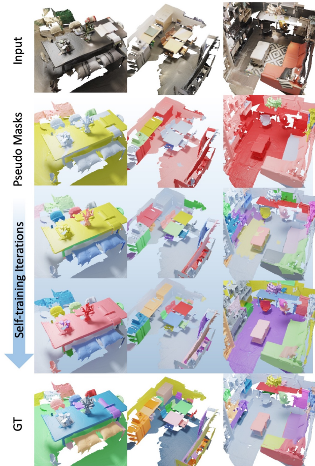
Figure 6. UnScene3D employs self-training to refine the initial sparse set of proposals. We can see consistent improvement over both the number of predicted instances and the quality of the instance masks. Here we show results using the pseudo annotations obtained from both modalities.
