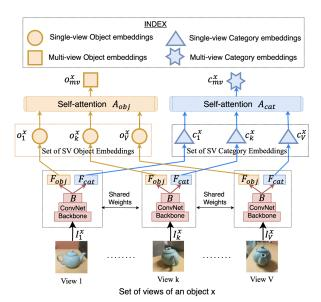
**Figure 3.** The Pose-invariant Attention Network (PAN) takes a set of multi-view images of an object as input, producing both single-view and multi-view embeddings for each representational subspace. The object embeddings are depicted in orange, while the category embeddings are in blue.
