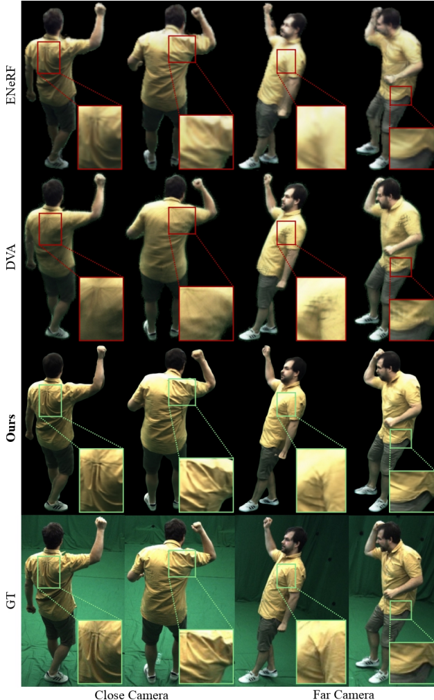
Figure 7. Comparison with Image-driven Approaches. ENeRF [17] produces artifacts under far views and DVA [28] suffers from blurred renderings. In contrast, our method generalizes well to far views and produces sharp results.
