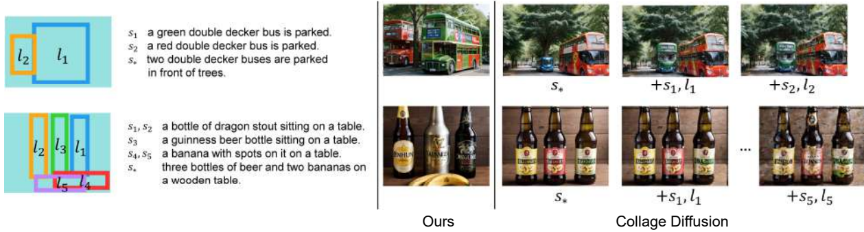
Figure 4. Comparison of generated images and their generation process by NoiseCollage and Collage Diffusion[31].
