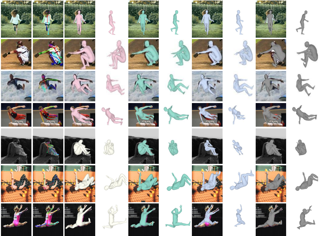
Figure 4. Body model fitting results. Pink: Regression (ProHMR [28]). White: Regression (HMR 2.0 [13]). Green: Regression + ScoreHMR (ours). Blue: Regression + ProHMR-fitting [28]. Grey: Regression + SMPLify [2].
