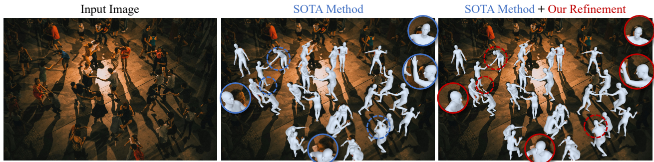
Figure 1. Although achieving remarkable 3D human reconstructions, a recent state-of-the-art monocular regression approach [13] may encounter challenges in aligning the human body model to the image (middle image). To address this, we propose an iterative refinement approach that utilizes image observations (e.g., 2D keypoint detections) and achieves better image-model alignment (right image).
