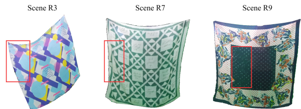
Figure 10. Optimizing the uv -map leads to some artifacts (red boxes) in the texture which are most noticeable when the texture contains regular geometric structures like straight lines or dots.
