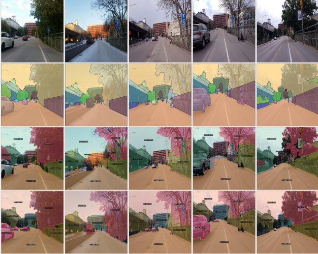
Figure 6. Examples of the change-aware sequential instance segmentation results (from top to bottom: input images; ground truth; results from Mask2Former and CTVIS). Objects with the consistent IDs share the same mask colors within each sequence.
