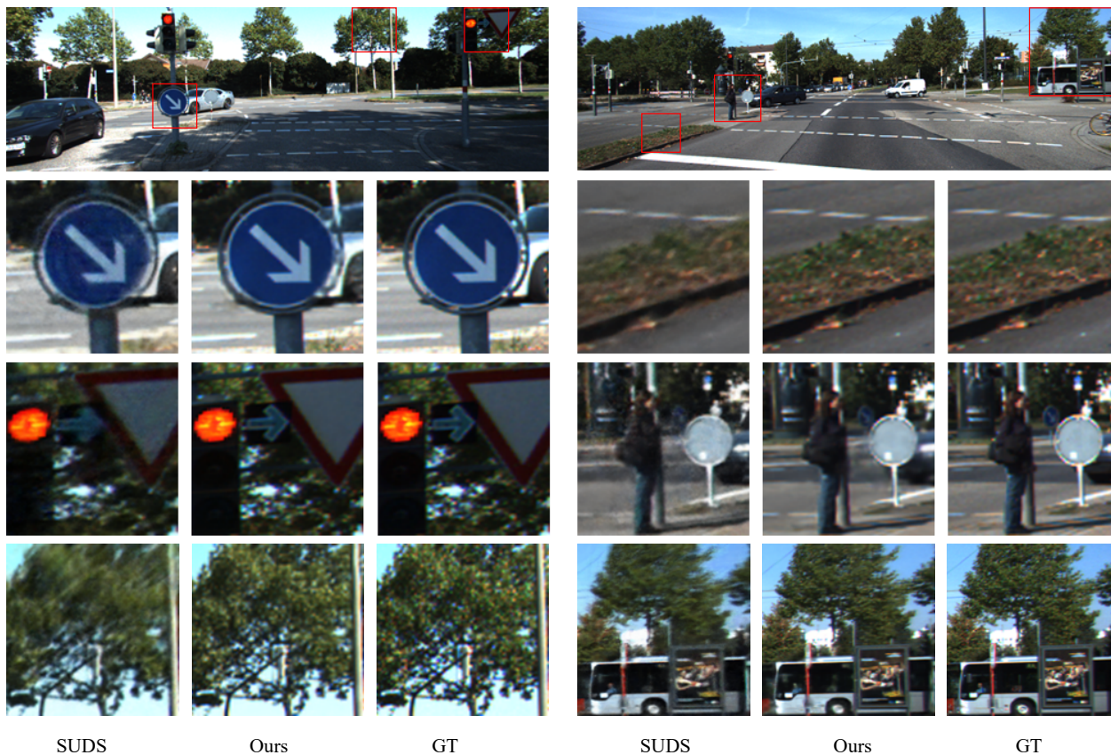
Figure 4. Image reconstruction on KITTI dataset. The first row is a sample of two scenes from the KITTI dataset. The following rows are some local details of the reconstruction results of the SUDS algorithm, our algorithm and the ground truth. Previous work failed to reconstruct some details and the image is a bit blurry. Our algorithm can achieve better reconstructed image quality and recover clearer details.
