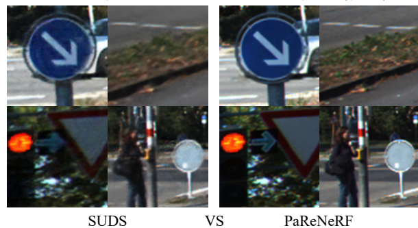
Figure 1. Comparison of image reconstruction performance on KITTI dataset. We show some local details of the image reconstruction results of the SUDS method and our PaReNeRF method. SUDS, the state-of-the-art neural rendering method for large-scale dynamic scenes, faces the problem of long training time and inference time, while PaReNeRF can generate higher-quality rendered images and significantly reduce training time (by 60%) and inference time (by 87%).
