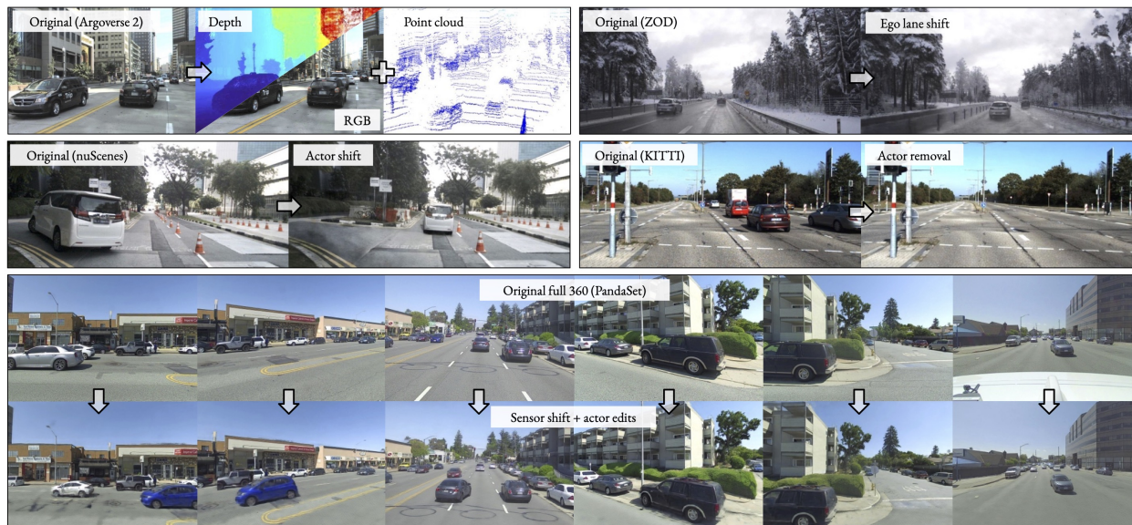
Figure 1. NeuRAD is a neural rendering method tailored to dynamic automotive scenes. With it, we can alter the pose of the ego vehicle and other road users as well as freely add and/or remove actors. These capabilities make NeuRAD suitable to serve as the foundation in components such as sensor-realistic closed-loop simulators or powerful data augmentation engines.
