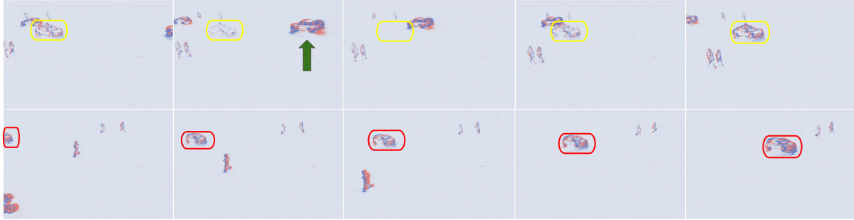
Figure 5. Demonstrating Effectiveness of Event Camera for Traffic Scenarios: Yellow circle (top row) tracks a car that halts at a stop sign with a lack of motion captured in the third frame, red circle (bottom row) tracks a car that violates the stop sign where motion is continuously captured in every frame. Additionally, a green arrow (top row) shows a car traveling at a high speed, resulting in a high event density.
