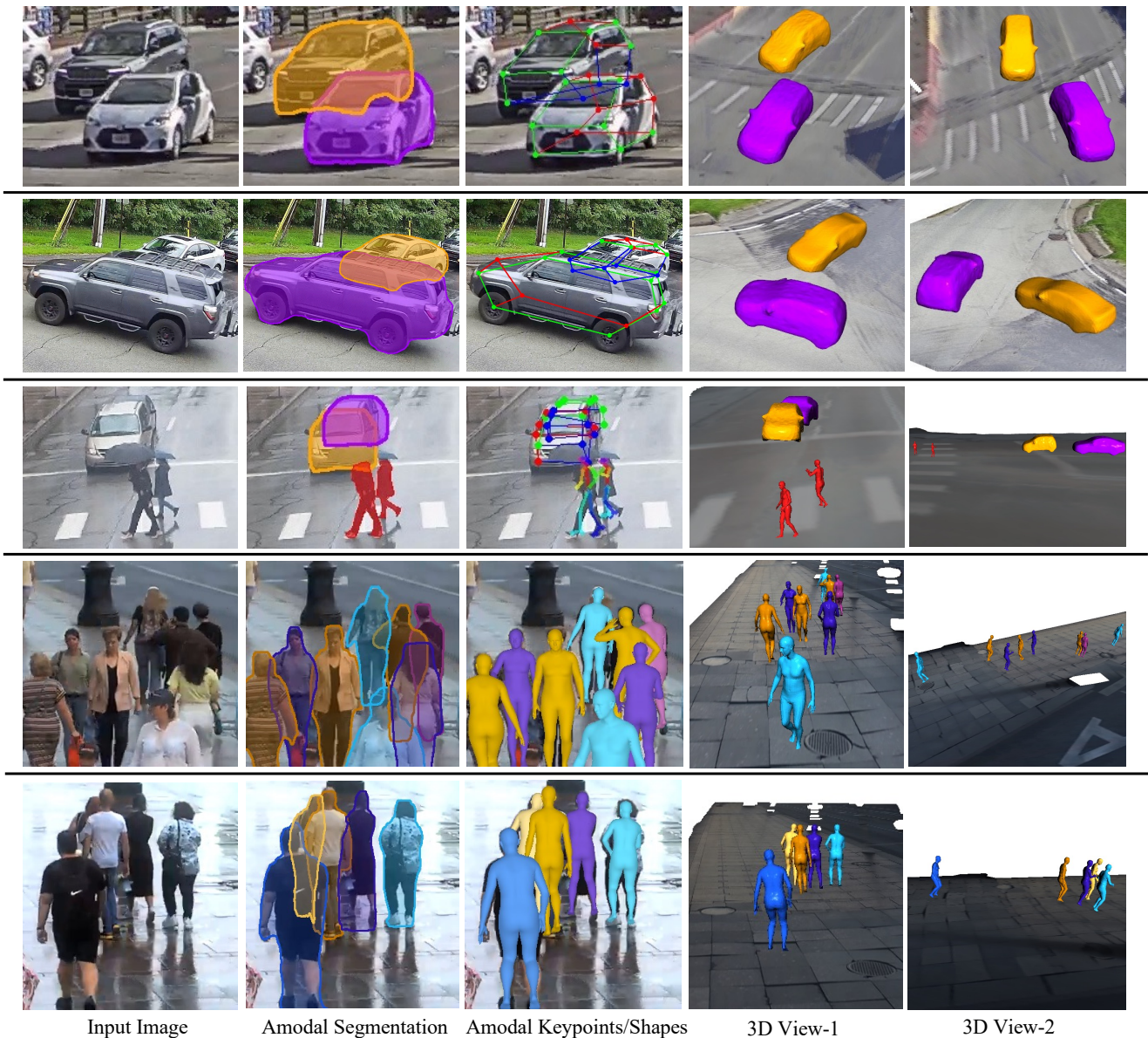
Figure 10. We show qualitative results of our method on real data. Our method produces accurate amodal segmentation, keypoints, as well as 3D poses and shapes across diverse poses and occlusion configurations. In particular, we show results on different level and types of occlusions like vehicle-vehicle ( row 1, 2, 3 ), vehicle-people ( row 3 ), and people-people occlusion ( row 4, 5 ).
