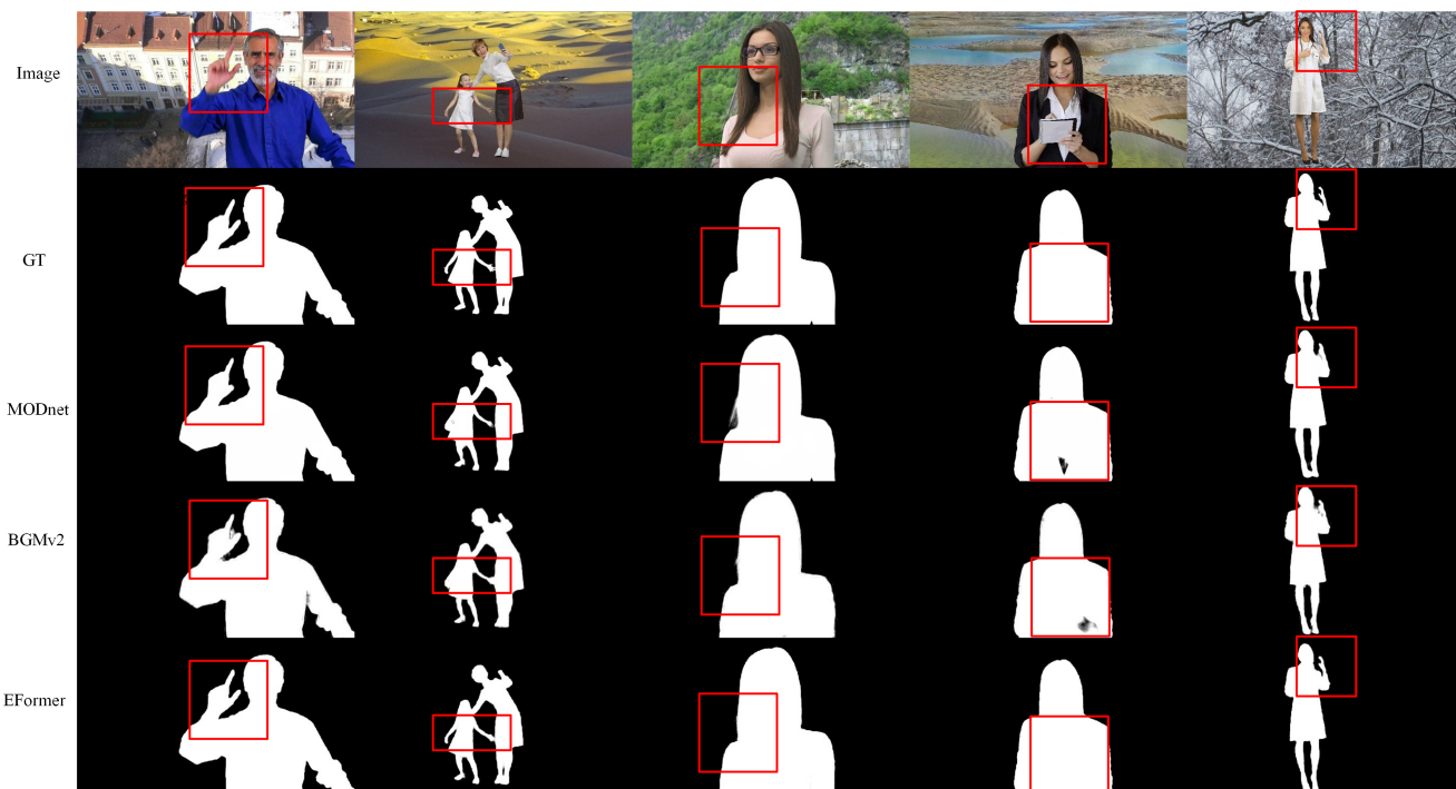
Figure 4. Visualization of portrait matte predictions from MODnet, BGMv2, and EFormer under challenging image from the test set of VideoMatte240K (JPEG SD Format). Our model shows a better ability to distinguish ambiguous foreground contours, as indicated by the red box. Please zoom in to view the detailed information.
