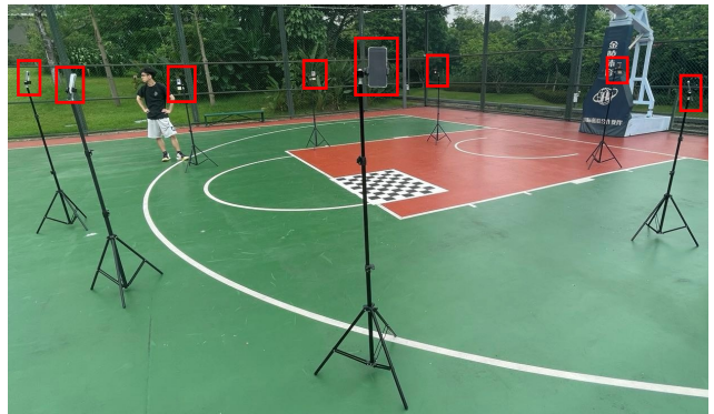
Figure 2. Equipment setting of data collection using 8 cameras. Cameras are attached to tripods.
