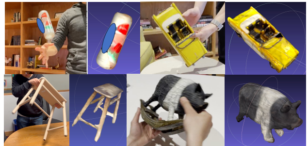
Figure 7. 3D-fy objects in-the-wild. (left) Videos of hand-manipulated objects; (right) we run ICON on the masked video to get poses+NeRF, and then use Marching Cubes to create meshes.
