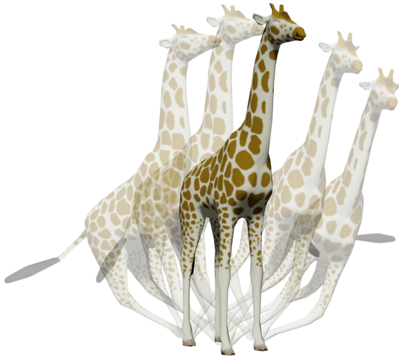
Figure 1. Visualization of our nonlinear subspace on a giraffe model discretized with tetrahedron finite elements. Overlays correspond to different frames from a selected neural mode.
