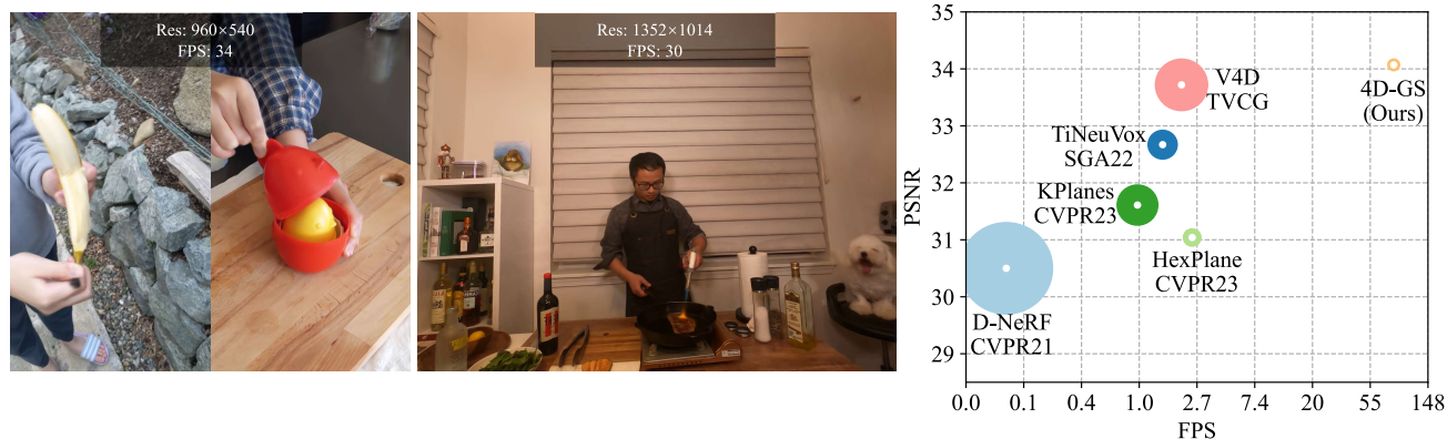
Figure 1. Our method achieves real-time rendering ‡ for dynamic scenes at high image resolutions while maintaining high rendering quality. The right figure is tested on synthetic datasets, where the radius of the dot corresponds to the training time. “Res”: resolution.
