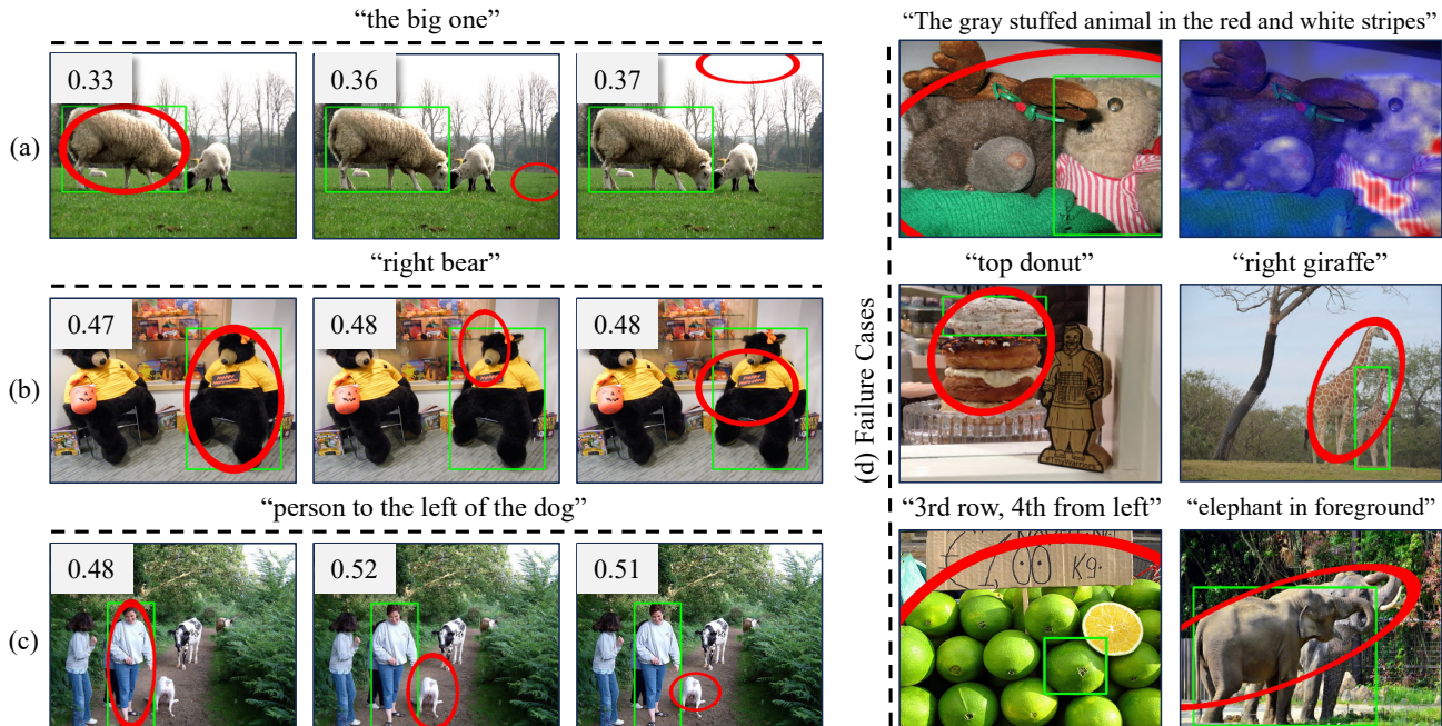
Figure 7. Illustration of scenarios where CLIP’s visual prompting falls short. We categorize three main scenarios: (a) high response to the background, (b) high response to inaccurate inclusion, and (c) high response to sub-words of expressions. The bounding boxes in green are the ground truth. Number on the left corner of the image is the matching score s(i^*, t) between visually prompted image i^* and text prompt t . The scores are the summation of two CLIPs, i.e. , ViT-B/16 and ViT-L/14.
