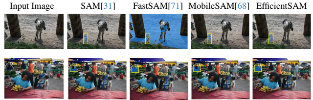
Figure 4. Visualization result on box-prompt input with SAM, FastSAM, MobileSAM, and our EfficientSAM model.
