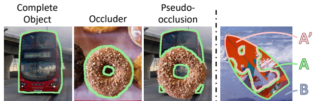
Figure 7. Left: We place complete objects on each other to create pseudo-occluded objects. Here, the bus is 66.2% occluded by the donut. Right: We can evaluate whether A' (formerly occluded) successfully completes the query object A by using pseudo-occluded objects and off-the-shelf metrics. But, these metrics do not assess whether A' \cup A fits into the background B . To this end, we conduct a user preference study to evaluate the generated objects in context.
