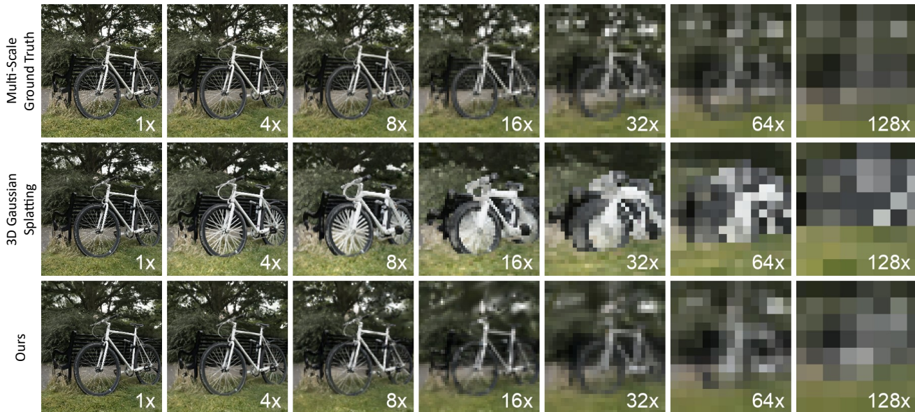
Figure 1. The rendering quality and speed of the original 3D Gaussian splatting[12] deteriorate severely at low resolutions or from distant cameras due to aliasing. Conversely, our multi-scale 3D Gaussians representation utilizes selective rendering to achieve faster (160% – 2400% at 4×-128× resolution) and more accurate rendering at lower resolutions.
