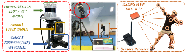
Figure 3. Portable Human Motion Capturing system.
