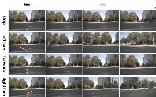
Figure 7. Task on action-conditioned prediction (simulation). Given the same starting frames and different future trajectories (shown in yellow dots in the first column), GenAD-act can simulate diverse futures following different ego intentions. More visualizations are in Appendix.
