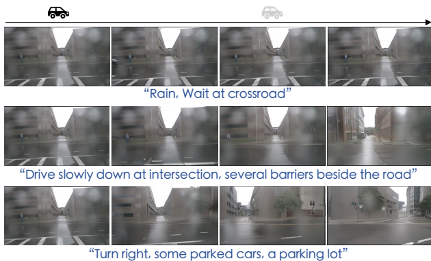
Figure 5. Task on language-conditioned prediction. Given two frames of a rainy scenario in the intersection and three high-level text conditions, GenAD simulates reasonable futures accordingly.
