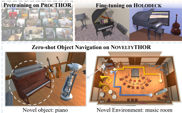
Figure 12. Zero-shot object navigation in novel scenes. Given a novel scene type, e.g., Music Room , HOLODECK can synthesize new scenes for fine-tuning to improve the performance of pretrained agents in expert-designed environments.
