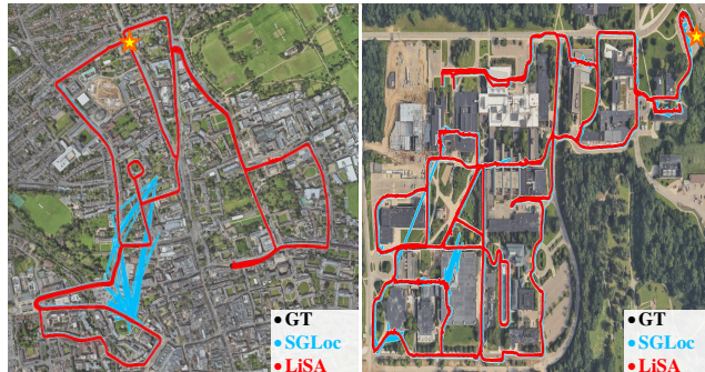
Figure 1. Teaser. This work studies the problem of LiDAR localization. We propose a novel method LiSA, which equips LiDAR localization methods with semantic awareness. We show the ground-truth and predicted trajectories on Oxford (left) and NCLT (right). Compared to the baseline method (SGLoc), LiSA achieves a much higher average localization accuracy and has much fewer catastrophic failures, without introducing extra computation or network parameters during inference.
