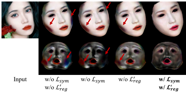
Figure 11. Effect of loss functions. In the refinement process for our StyleGAN2 model, without loss functions \mathcal{L}_{sym} and \mathcal{L}'_{reg} leads to over-fitting of the input image, resulting in artifacts.
