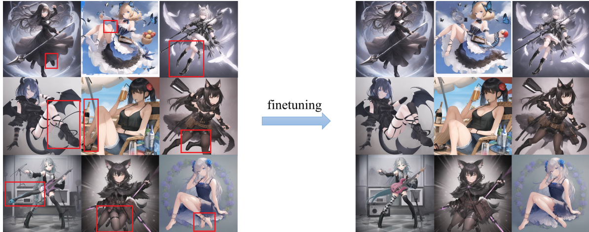
Figure 6. Image samples of the pre-trained model and the fine-tuned model. The images on the left side of the arrows are distorted images (such as having 3 legs in the image) generated by the pre-trained model, while the images on the right side are normal images generated after fine-tuning the model. Both sets of images used the same initial Gaussian noise, prompts, and seeds.
