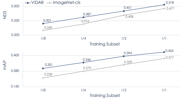
Figure 6. Validation of ViDAR on Fine-tuning with limited supervised data. We verify ViDAR on supervision efficiency by reducing available annotations for 3D object detection during downstream fine-tuning (from the full training set to a 1/8th subset) and observe a continuous improvement on each subset.
