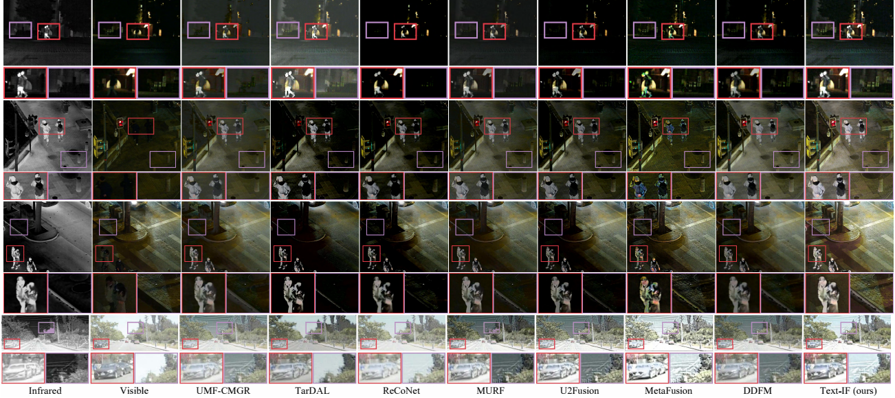
Figure 3. Qualitative comparison of our Text-IF without text guidance (without additional semantic information) and existing image fusion methods. From top to bottom: data from MSRS, two groups of data from LLVIP, and data from RoadScene datasets, respectively.
