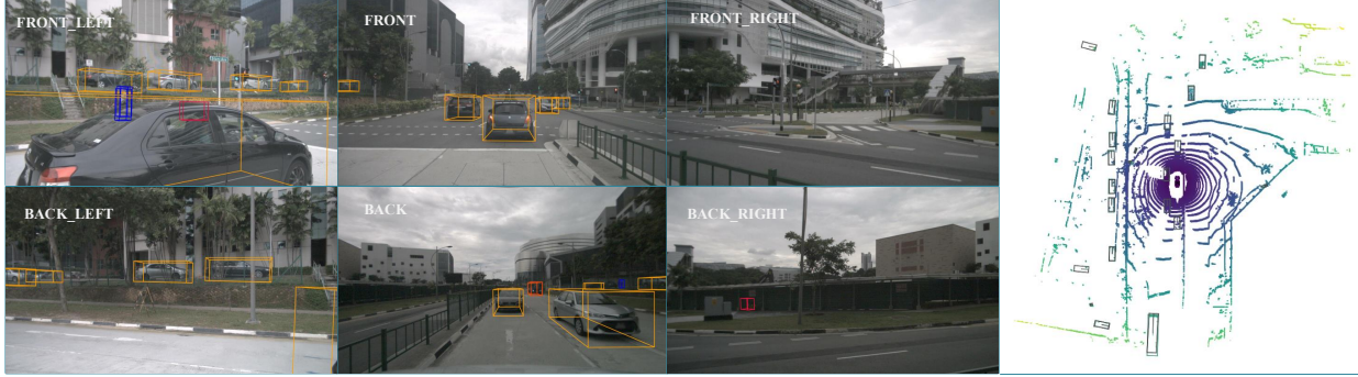
Figure 5. Examples of 3D object detections on nuScenes validation set. We visualize the 3D bounding boxes of car, pedestrian and bicycle with orange , blue and red colors in the multi-view images. In the point cloud, the predictions are in gray and GTs are in green .
