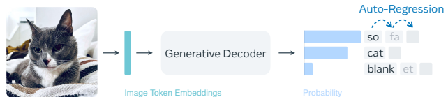
Figure 1. Object recognition as next token prediction using a generative decoder such as a transformer-based language model to auto-regressively predict object labels. Photo authorized with CC BY 4.0.
