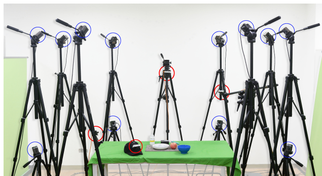
Figure 3. Capture platform. 12 MoCap cameras are circled in blue and 4 RGB cameras in red.
