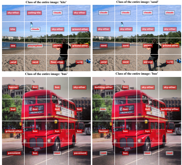
Figure 2. The left side of the figure presents the original CLIP’s classification results for a 4 \times 4 grid of regions, demonstrating that CLIP can capture more granular classification information within the image. The right side shows the results of the trained CLIP-RC encoder for classifying the same 4 \times 4 grid of regions. By our design, both seen and unseen classes achieve more accurate classification. Note, the red tags indicate unseen classes.
