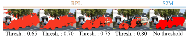
Figure 2. Existing anomaly score-based OoD detection method such as RPL [32] is sensitive to the thresholds while S2M eliminates the need for threshold selection , which is more practical. Besides, S2M also gives a more precise mask.
