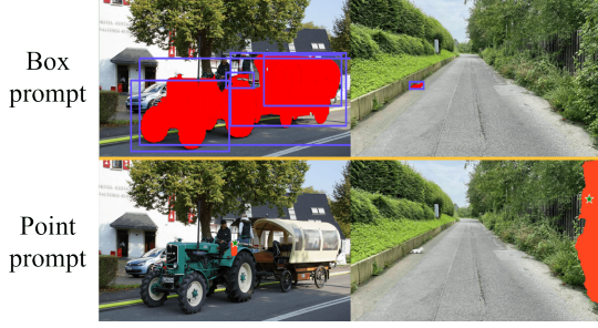
Figure 4. Box prompts can lead to more accurate segmentation for the OoD objects compared to point prompts. We derive point prompts from the locations corresponding to the extreme values of the anomaly scores. Visual analysis indicates that box prompts substantially improve the model’s tolerance to noise. We employ all generated box prompts to obtain a comprehensive mask of the OoD object, which ensures that the entire object is covered.
