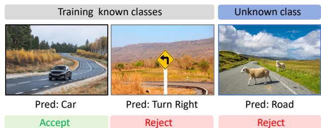
Figure 1. Illustration of typical failure cases arise when deploying models in real-world applications: misclassified example from known classes (e.g., recognize Turn Left as Turn Right), and semantic-shifted OOD example from unknown classes (e.g., sheep). A unified failure detector should accept correctly recognized examples and reject both misclassified and OOD examples.
