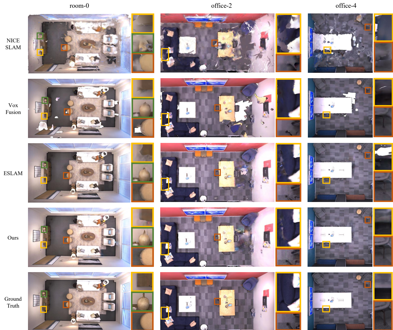
Figure 4. Qualitative comparison on scene reconstruction of our method and baseline. The ground truth images and details are rendered with ReplicaViewer software [38]. We visualize 3 selected scenes of Replica dataset [38] and details are highlighted with colorful boxes. Our method achieves more accurate detailed geometry and higher completion, especially in places that have limited observations.
