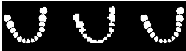
Figure 6. Comparison of Bilinear Interpolation to Permutation-based Upscaler. (left) Ground Truth, (middle) Bilinear Interpolation, (right) Permutation-based Upscaler.
