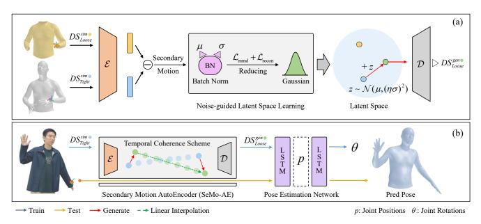
Figure 3. Overview of Loose Inertial Poser. (a) The training process of SeMo-AE and how it generates loose-wear IMU data from tightwear IMU data. (b) The training of the pose estimation model and how it performs pose estimation. We generate diverse loose-wear IMU data using SeMo-AE and Temporal Coherence Scheme to train the pose estimation model, making it suitable for our loose-wear jacket.
