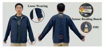
Figure 2. Prototype demonstration of the loose-wear jacket embedded with IMU sensors and the circuit board for data collection.
