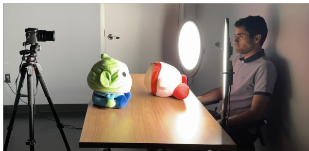
Figure 2. Capture setup. We illuminate the objects of interest with two area lights to ensure that sufficient amount of light is reflected off the eyes.
