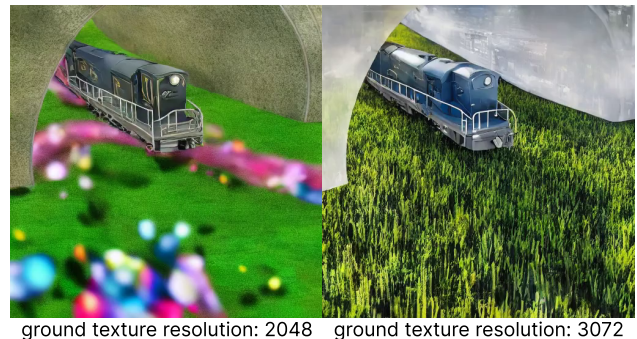
Figure 7. Effect of different texture resolution. If the ground’s texture resolution is too low ( 2048 \times 2048 ), artifacts appear at ground regions in the final rendered image compared with using a higher texture resolution ( 3072 \times 3072 ). Prompt: a train running in a field of green grass.
