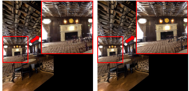
Figure 10. Warping with and without super-resolution. (a) The phenomenon in Fig. 9 causes blurry warping. (b) With super-resolution, we can significantly enhance the sharpness of the warped image.
