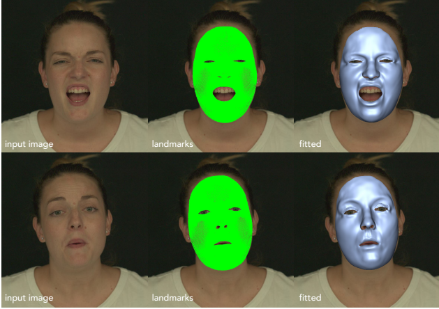
Figure 13. We demonstrate a proof of concept of the application of our model in face reconstruction, where our AIM model can be fit to 2D landmarks obtained from a pre-trained landmark detector, capturing both the pose and expression of the person faithfully.
