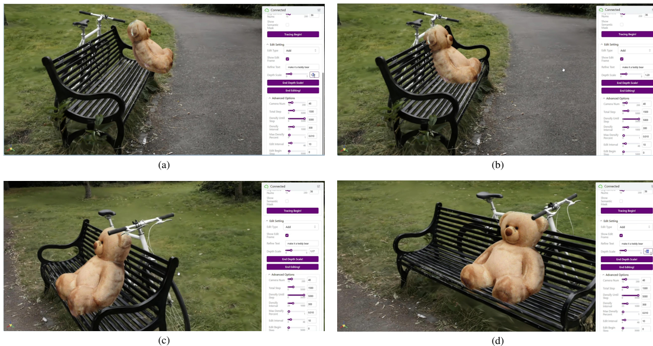
Figure 2. Object Incorporation with WebUI. Empowered by our interactive WebUI, the depth scale addresses the limitation of monocular depth estimation, which cannot guarantee precise depth map predictions. As can be seen in (a), inaccurate results can lead to failures when aligning generated objects with Gaussian scenes. We leverage the interactive nature of our WebUI to dynamically adjust the estimated depth in real-time, thus resolving this issue, demonstrated in other images.
