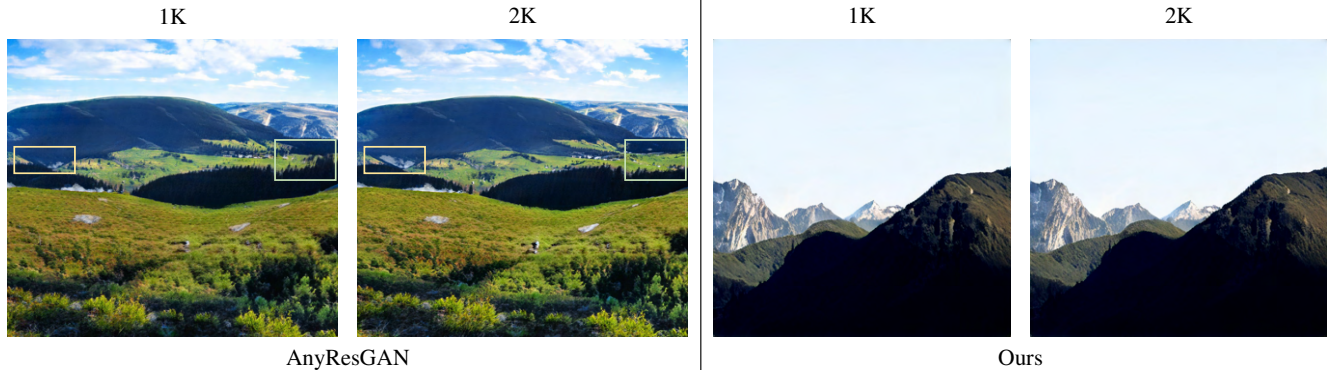
Figure 3. Scale consistency of our CLIF renderer. In each pair, the left is rendering at resolution 1K, the right is rendering at resolution 2K then downsampling to 1K. Yellow/green boxes show two examples of inconsistent areas in AnyResGAN (besides the boxes, the object boundary also does not align for 1K/2K of AnyResGAN).
