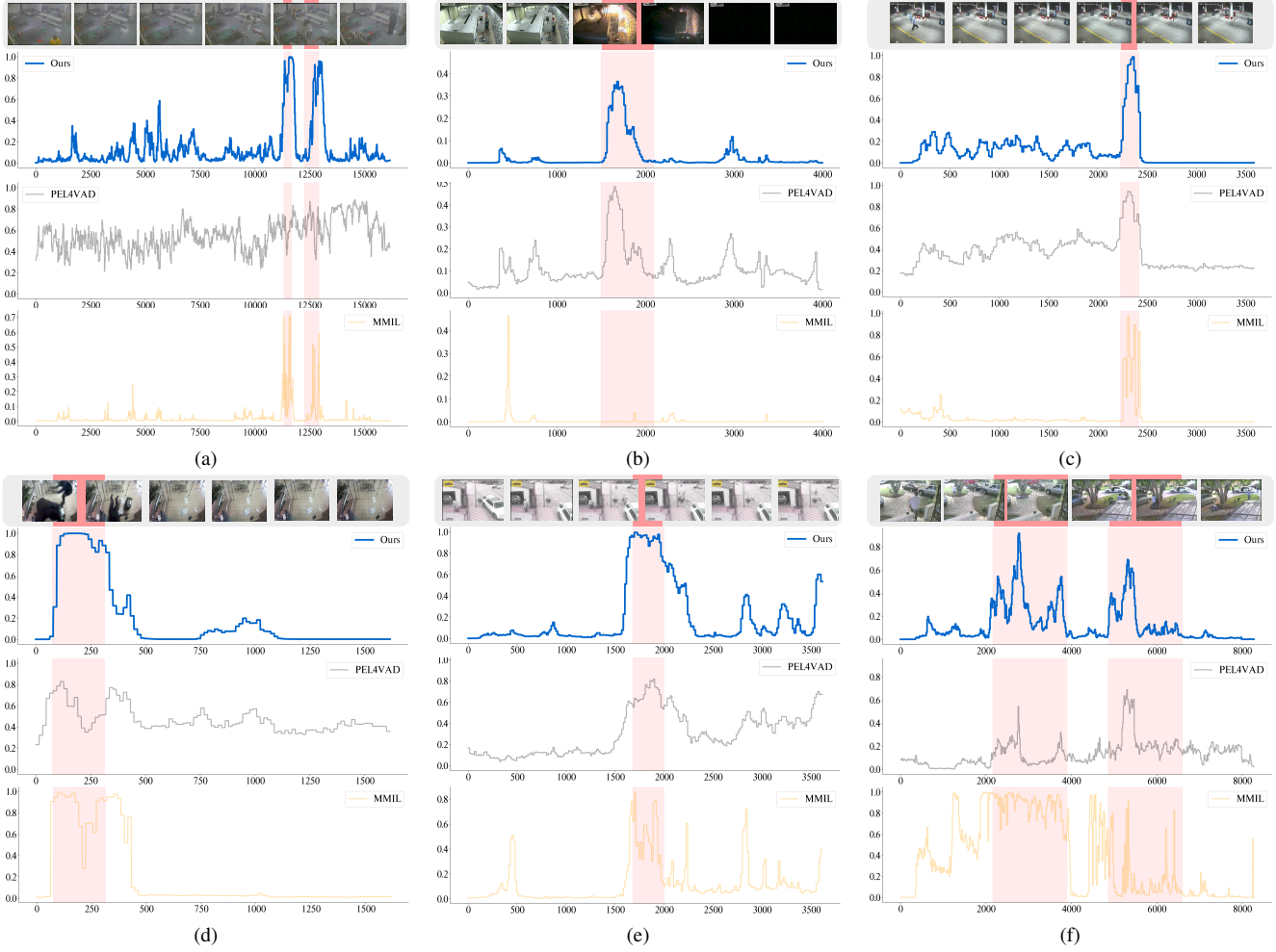
Figure 2. Anomaly scores of abnormal videos on UCF-Crime. The Y-axis represents anomaly scores (1 for abnormal and 0 for normal), while the X-axis represents the frame number of videos. The pink area refers to the regions where anomalies take place. The blue lines are the predictions of our method; the gray lines are the predictions of PEL4VAD [7]; the orange lines are predictions of MMIL [9]. The above frames are snapshots from videos and the red ranges indicate the abnormal sections.
