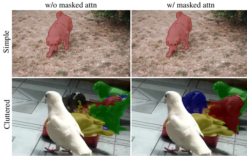
Figure S3. Comparisons of Cutie with/without masked attention. While both work well in simple cases, masked attention helps to differentiate similarly-looking objects.
