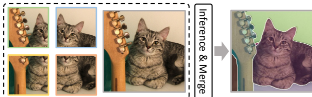
Figure 2. Illustration of the patch inference. During inference, we divide the input image into patches, thereby increasing the effective resolution.
