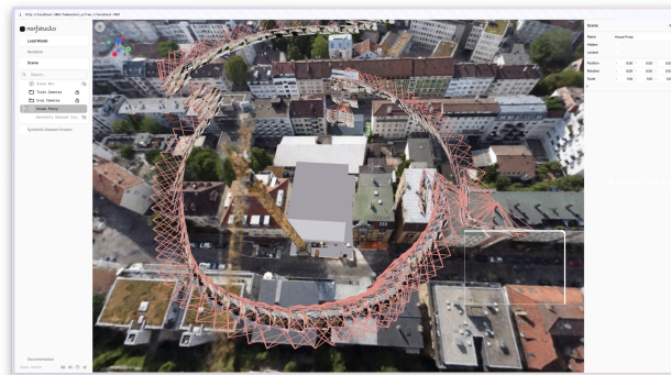
Figure C2. Viewer – Outlining the placement of a proxy object within an existing NeRF scene. The viewer is divided into a 3D viewport at the center, a scene and selection column on the left and a selection specific control column on the right.
