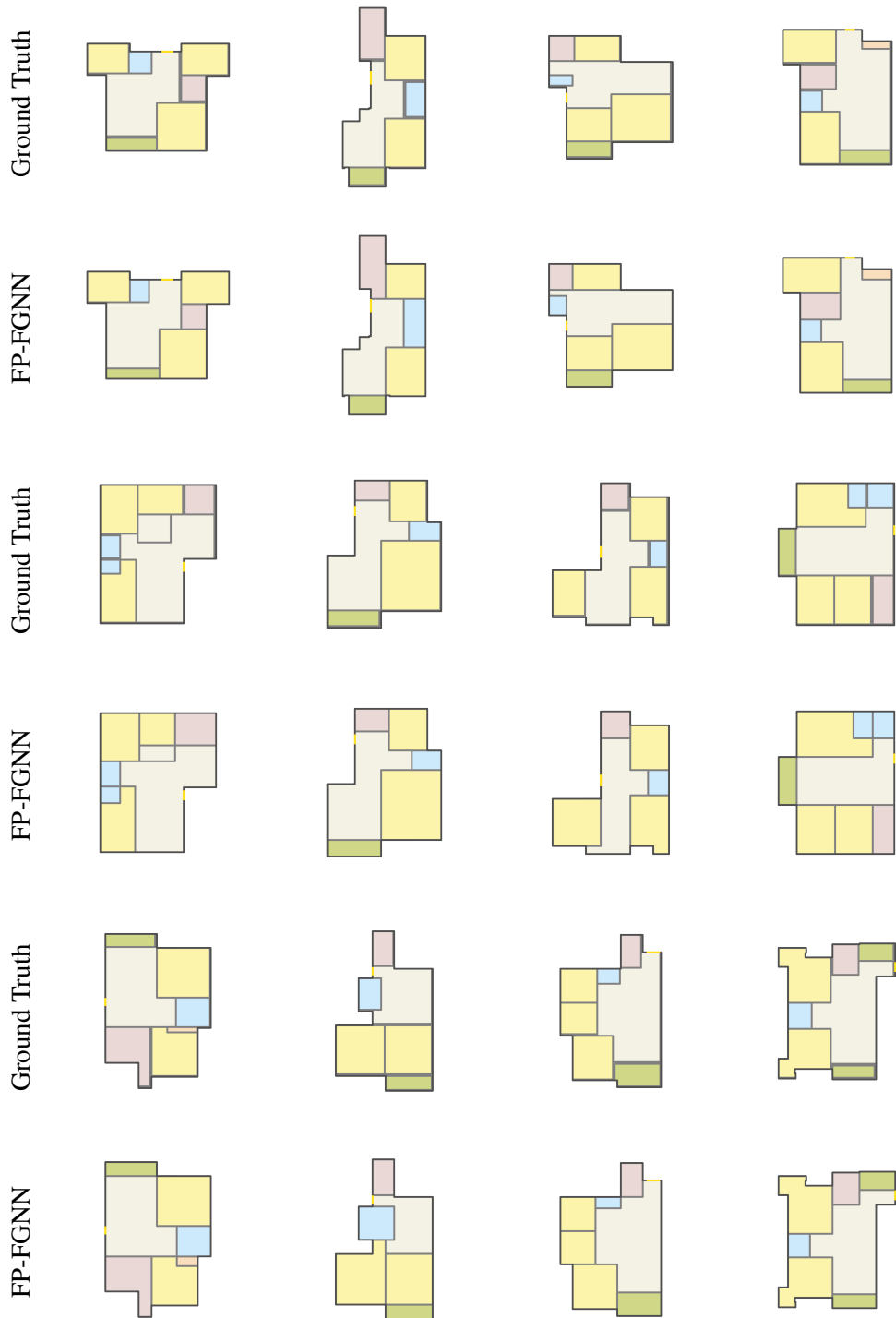
Figure 10. Comparison of floorplans generated by FP-FGNN with the ground truth after post-processing.
