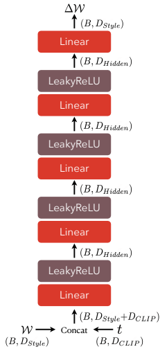
Figure 1. Architecture of the StyleEntity Mapper, where D_{style} represents the dimension of StyleGAN’s style space, D_{CLIP} denotes the CLIP space dimension, and D_{hidden} is the dimension of the MLP’s hidden layers.
