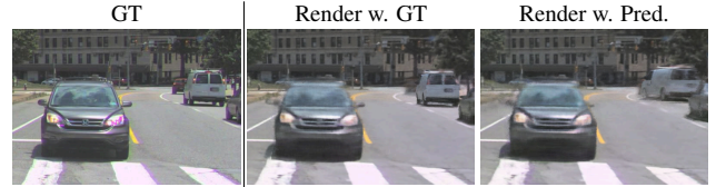
Figure 10. Failure case of predicted 3D bounding boxes. While the car in the foreground is well reconstructed with both ground truth and predicted 3D bounding boxes, the van in the background is rendered with incorrect orientation and is slightly too big.
